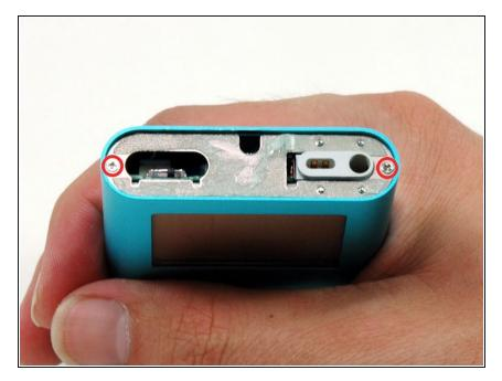
• Remove the two #00 Phillips screws securing the headphone jack to the casing.
