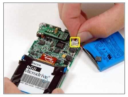
• Carefully disconnect the battery from the logic board. Make sure to pull only on the connector and not on the battery wires.
