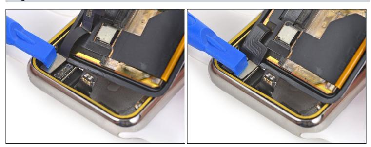
Use a plastic opening tool to reconnect the display data and digitizer cable connectors.
