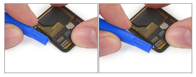
Use a plastic opening tool to scrape adhesive off the back of the screen.
