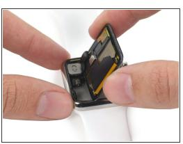
Fold the screen up and over to the right, to expose the cables underneath.
