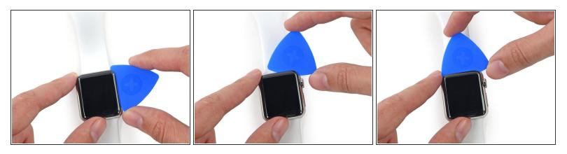
Work the pick around the top right corner, and roll it along the top edge of the screen.
