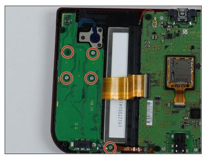
Next, locate the five 3mm screws on the left board and remove them using a JIS #000 screwdriver.
