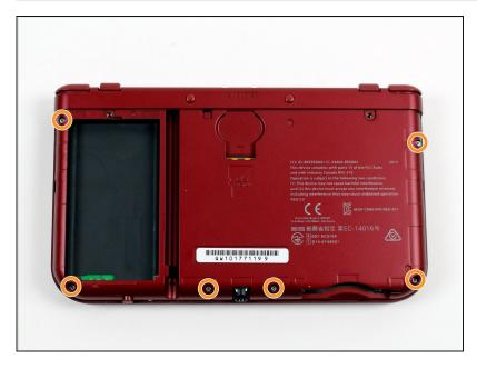
Remove six 6mm screws on secondary panel using a JIS #000 screwdriver.
