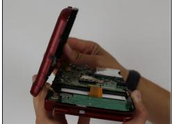
① To pry off the cover, carefully lift it up and away from the hinges (in order to clear the headphone port), then pivot it towards the hinges to expose the circuit boards.
