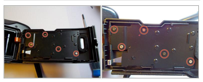
Remove the five screws circled in red from the plastic on the back of the camera.
