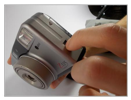
Push down on the black switch located on the side of the camera.
