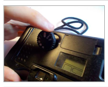
With the screw holding it in place removed, the mode selection wheel should come right off. Simply remove it from its socket.
