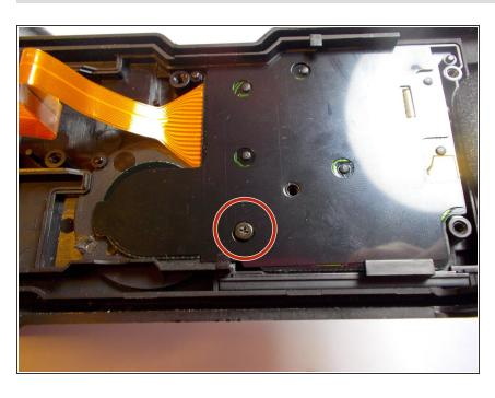
You should now see the a strip of black plastic covering the back of the display's logic board. Remove the screw circled in red.
