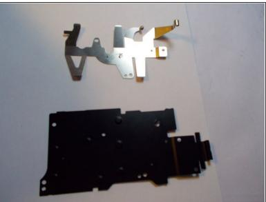
Pull on the metallic piece that is sticking out from underneath the plastic. This will allow you to remove both the piece of black plastic and the metallic piece from the camera.
