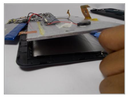
Work the spudger all the way around until the LCD is free from the screen holder.
