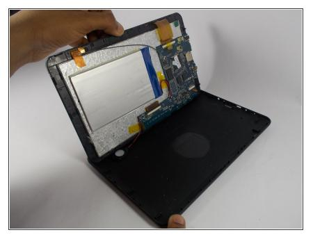
• Once the screen has fully separated from the back of the tablet, gently lift up the edges to remove the screen.
