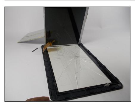
• Finally, lift the LCD off, removing it from the screen holder and the motherboard.
