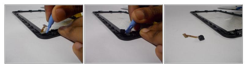
• Use the smaller plastic opening tool to remove the camera from its socket.
