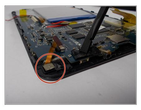
Remove the tape covering the front facing camera entirely to expose one of the motherboard screws.
