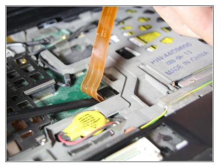
• Disconnect the ribbon cable with the spudger.
