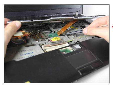
• With the panel disconnected, lift the keyboard.
