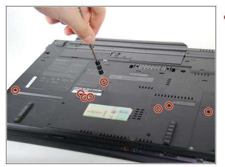
Remove the eight 14mm screws using the Phillips #0 Screwdriver.
