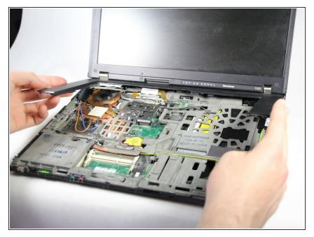
• Remove the speaker cover by carefully pulling up and towards you.
