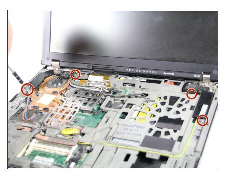
Remove the four 3mm screws on the speakers with the Phillips #0 Screwdriver.
