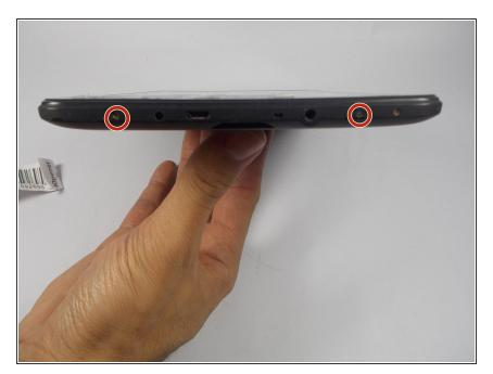
Using a #00 Phillips head screwdriver, remove the two 5.4mm bottom screws.
