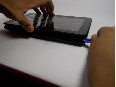
Insert a plastic opening tool between the screen and the rear case and gently work your way around the tablet.
