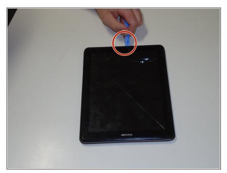
Pry open the tablet by having the tablet face upward. To pry open, start over in the left corner (by the buttons) working clockwise until the tablet is open.
