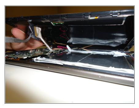
Remove the silver cable by removing the tape that connects the cable and screen. Gently detach the gold cable from the outlet.
