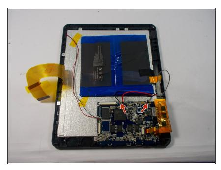
Cut red, black, and gray wires connecting the battery to the motherboard.
