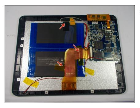
Remove tape on top of battery.
