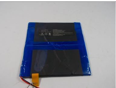
Use the plastic opening tool and the spudger to pry up and remove the battery.
