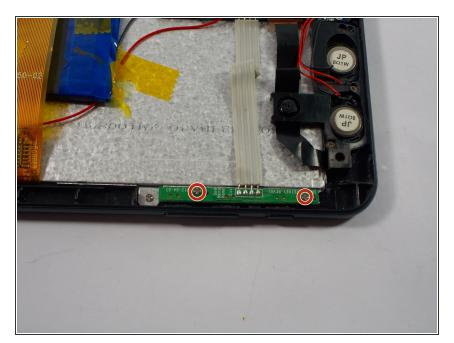
Remove 2 silver 4 cm Phillips screws in the top right side of the device.
