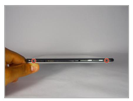
Remove 2 black 4 cm Phillips screws on either side of the bottom of the device.
