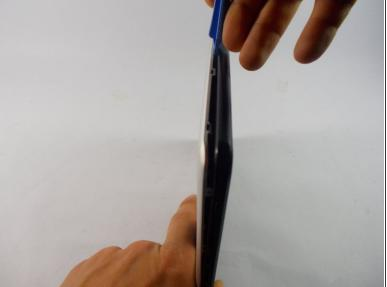
Use the plastic opening tools and the spudger around the outside of silver metal back plate on the device to pry off the back plate.
