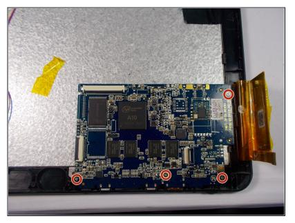
Remove 4 silver 4 cm Philips screws holding down the motherboard.
