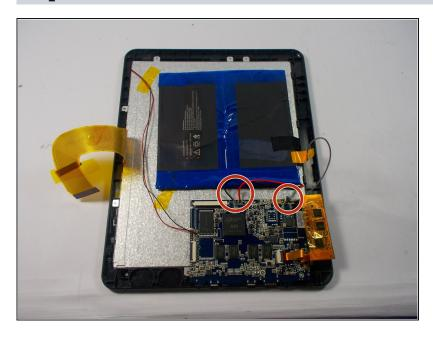
Cut red black and gray wires attached to the bottom of the motherboard connecting to the battery.
