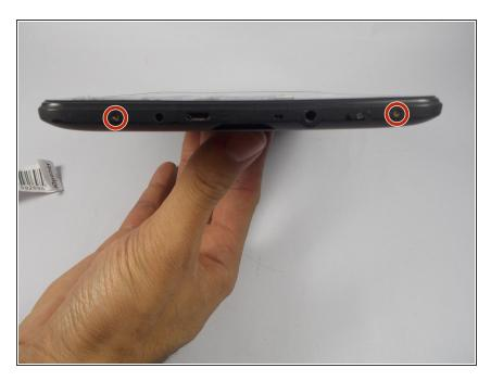
• Using a Philips screwdriver, remove the two 2.44 mm screws from the back plate of the tablet.
