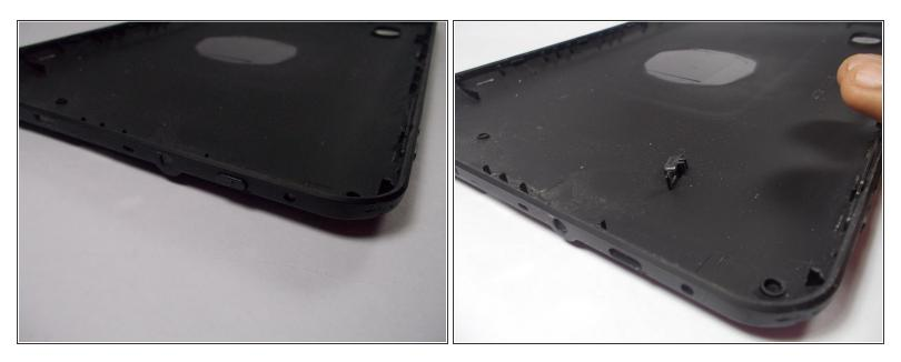
• Push on the old power button to remove it and install the new power button.
