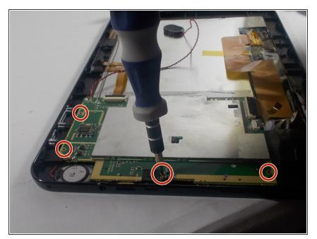
Locate and remove the four screws holding the motherboard on the device using the philips head screwdriver.
