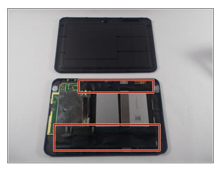
• Remove the electrical tape surrounding the battery.
