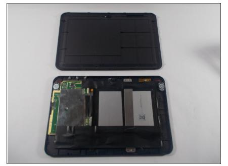
The back cover should then be able to easily be removed from the device and you should see the battery and other internal components.
