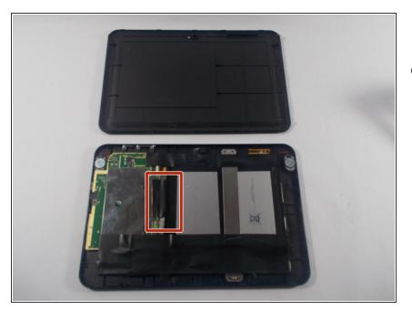
Locate and remove the copper tape connecting the motherboard to the back of the screen
