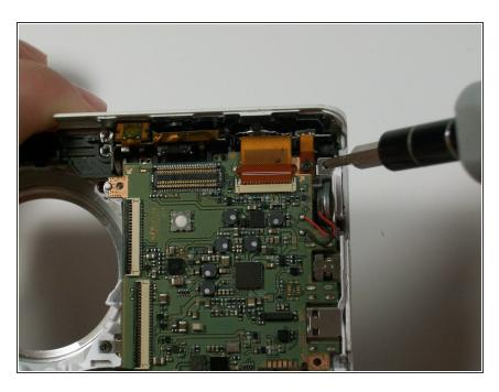
Remove the 2.381 mm screw that is holding the copper to the control board with a Phillips #00 screw driver.
