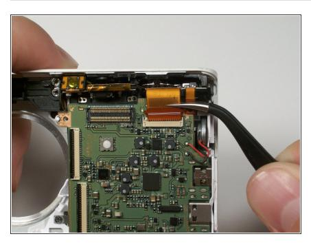
Use tweezers to pull copper connector from the control board.
