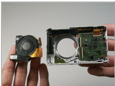
Remove the lens assembly from the camera.
