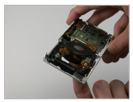
From the front of the camera, push the lens through the back of the camer.a
