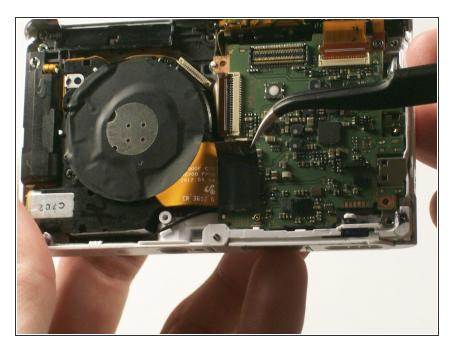
Use the tweezers to remove the black electrical tape covering the copper connector to the control board.
