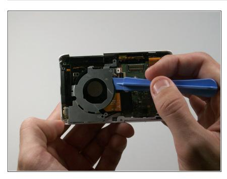
Use the plastic opening tool to remove the silver metal lens cover.
