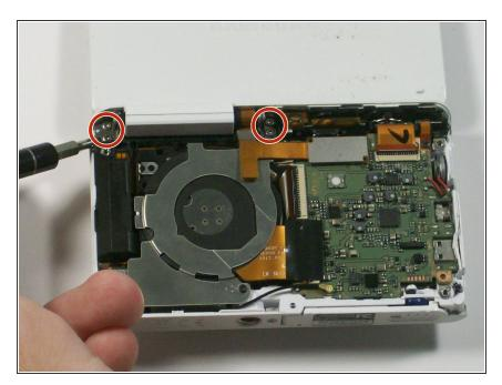
Use the Phillips #00 screw driver to remove the four 2.381 mm screws next to the screen hinge.
