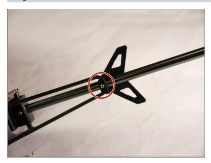
• Remove the 4 mm Phillips #00 screw from the tail.
