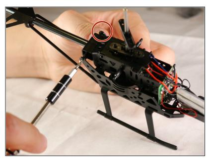
Remove the two 8 mm Phillips #00 screws between the motor casing and the body.
