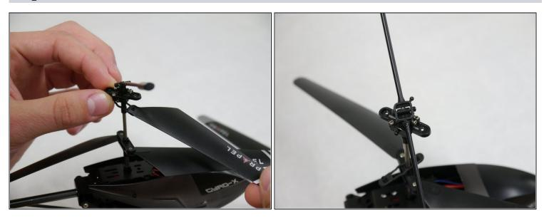
Pull the rotors away from the mounting brackets.
