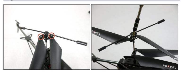
• Remove the two 6.0 mm Phillips #00 screws from the rotors.
