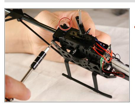
Remove the two 8 mm Phillips #00 screws between the motor casing and the body.
