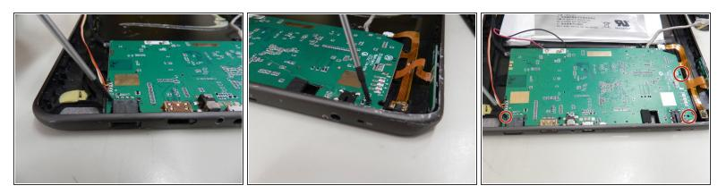
Using a Philips #00 screwdriver, unscrew the 3 screws that connects the motherboard to the tablet.
