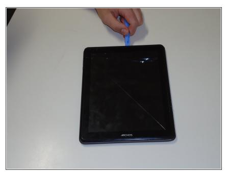
With the tablet facing you pry open the tablet. Start over in the left corner (by the buttons) working clockwise until the tablet is open using either a set of opening picks or a plastic pry tool.
