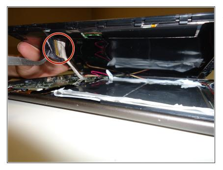
Now remove the silver cable by removing the tape connecting the cable and screen, then gently detaching the gold cable from the outlet.
