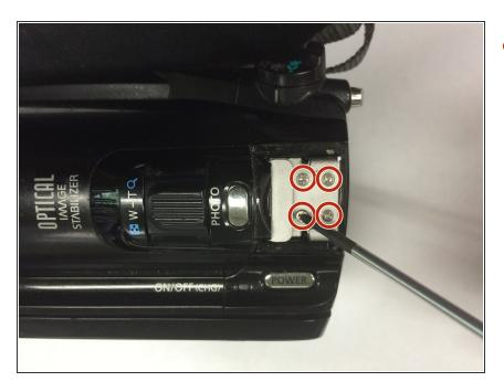
Unscrew the four 6 millimeter screws with the Phillips screwdriver.
