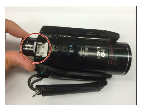
Remove the mini advanced shoe from the top of the camcorder.
