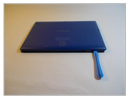
Place the plastic opening tool between the front and rear cover and pry up on each corner of the cover.
