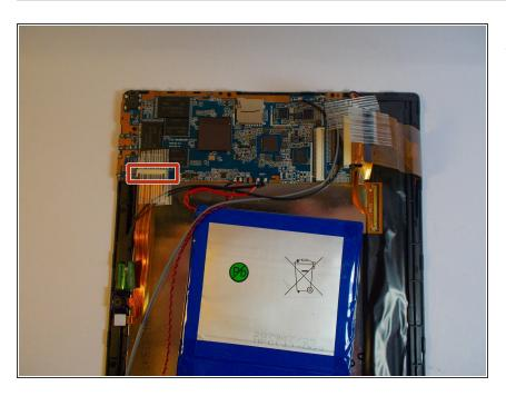
• Pull camera plug upward and away from the motherboard.
