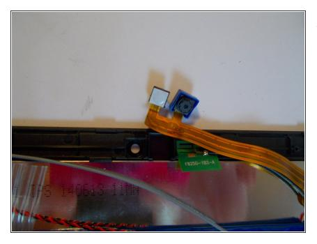
Remove each camera from the front cover assembly. They are simply held in by tension.
