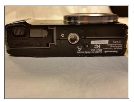
Remove the bottom Phillips head screws on the camera to take off the outer plastic housing. Be careful when pulling the piece off; if something seems stuck, double check to make sure every screw on the bottom was removed.
