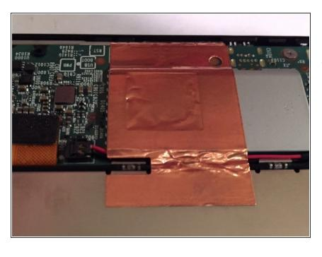
If your device has copper tape attached to the battery, carefully peel it off the battery.
