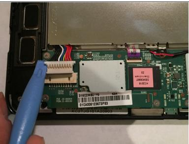
Detach the plastic piece that connects the wires to the motherboard using the plastic opening tool.
