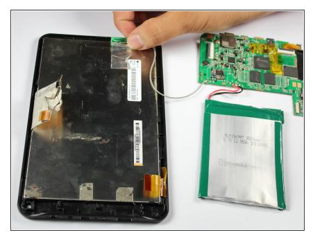
Carefully pry off the component that is taped to the LCD display at the top of the R1.
