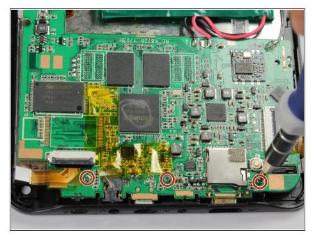
Remove the three 4 mm screws along the base of the motherboard with a Phillips #00 Screwdriver.
