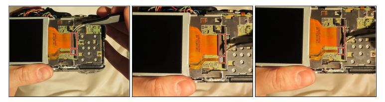
• Using the <u>tweezers</u>, lift the hinges connecting the two ribbon wires to the camera.
