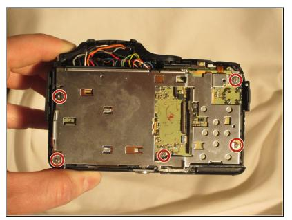
Remove these five Phillips screws, from the back of the camera, with the Phillips screwdriver.
