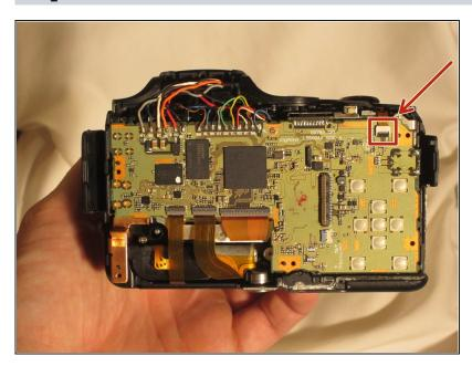
Using the pointed edge of the spudger, lift the hinge that secures this flex circuit. This will unfasten the flexible ribbon wire.
