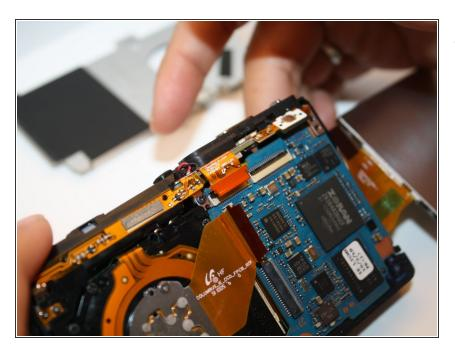
Slowly lift with your fingers, the top frame of the camera up, disconnecting it from the main piece.
