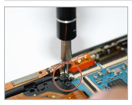
Remove the 4 mm Philip screws located above the center film strip with the Philip screw driver. This will allow the top frame to come loose to take off.
