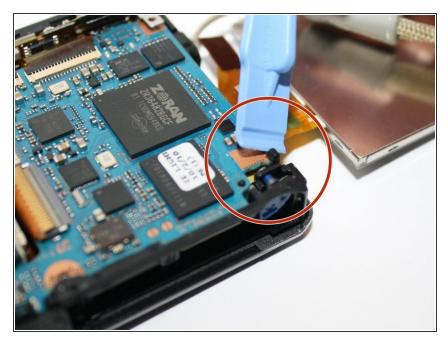
Then pull the black claw located at the bottom right of the camera, to the right with the plastic opening tool. This holds the main plate down.
