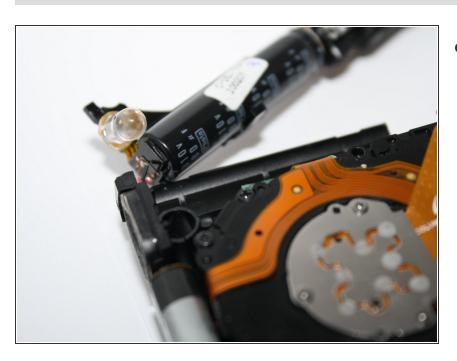
This piece disconnected exposes the light bulb that you can change out at this point in the guide.
