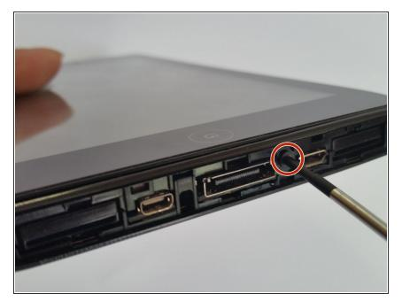
Remove the five 4 mm screws from the edges of the tablet with a Phillips #00 screwdriver.
