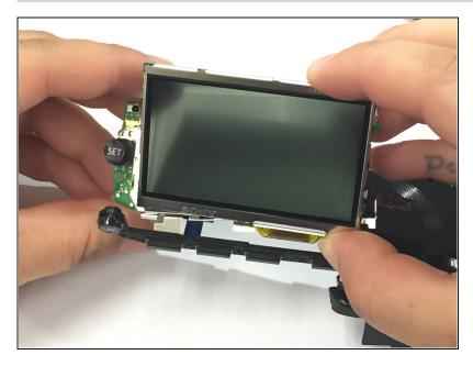
• Using your fingers, remove the LCD screen.
