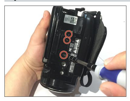
Turn the camcorder upside down and remove the three 3x4 mm Phillips screws securing the black plastic case.
