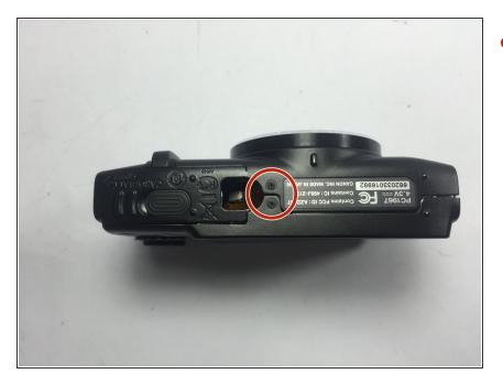
Using the same screwdriver, remove the two 3.4 mm screws on the bottom of the camera.
