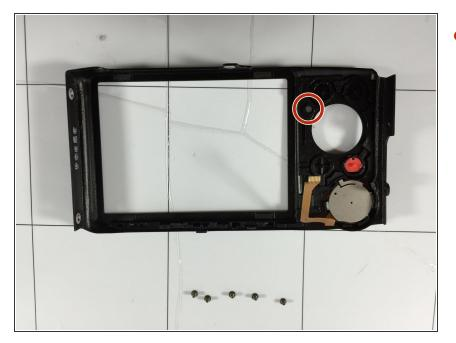
When removing the plastic casting, do not pull it all the way off. Detach the small tab first and make sure nothing else is attached to the casing.
