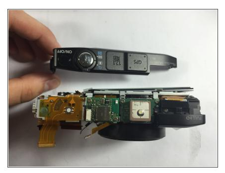
• Lift the small plastic tab, located on the front of the camera, to remove the GPS cover.
