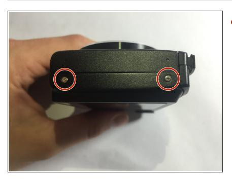
• Use a Phillips #00 screwdriver to remove the two 3.4 mm screws on the left side of the camera.
