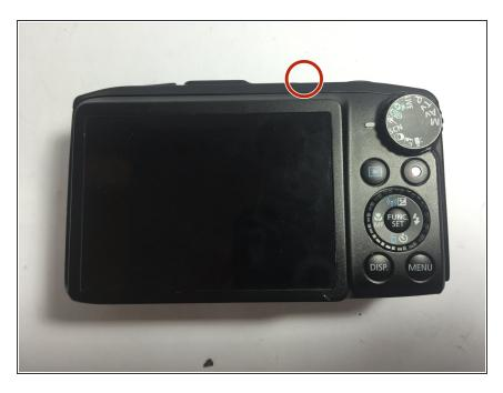
Turn off the camera by pressing and holding the ON/OFF button that is located on the top of the camera.
