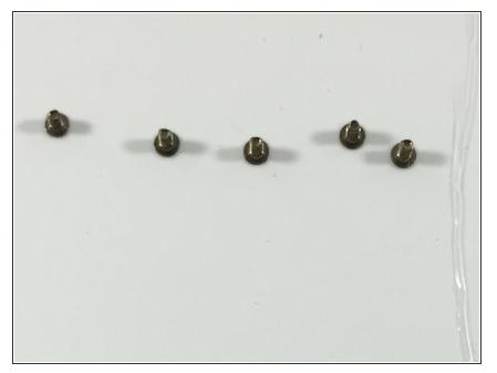
Now you can begin to take the outer screws out. Removing these will allow you to remove the camera case. It will require a #00 Phillips Screwdriver.
