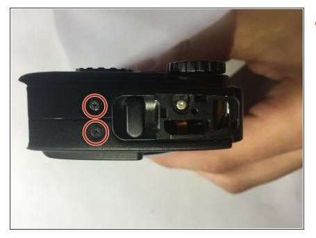
There are two screws to remove on the right side of the camera as well, as marked in the photo. Remove these screws next.
