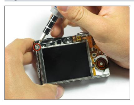
Remove the 1.75 mm Phillips #00 located at the top left of the LCD screen.
