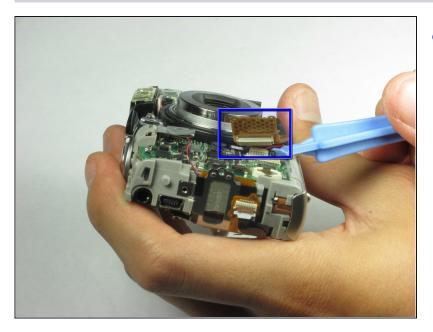
• Use a spudger or a flathead screwdriver to remove the camera lens cable located in the front of the camera.
