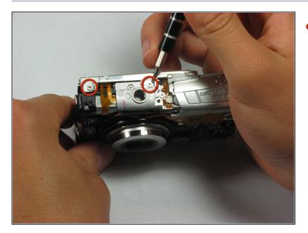
• Remove the two 3.4 mm Phillips #00 located at the bottom of the camera.
