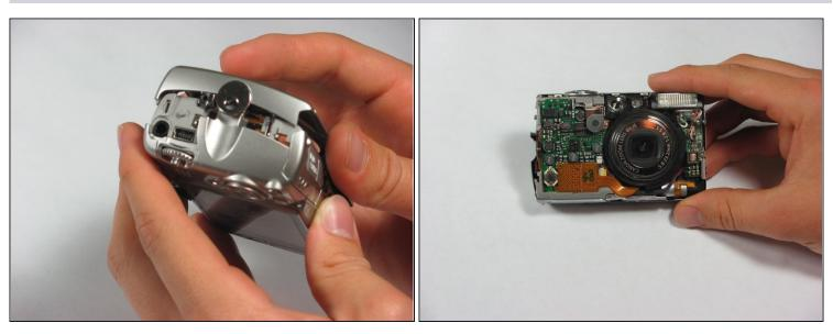
• Gently pull the front cover straight out from the camera. This will expose the wiring on the front of the camera.
