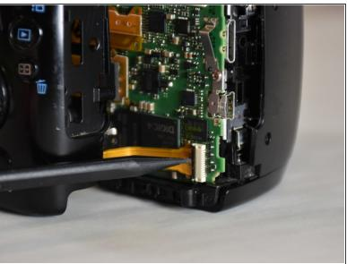
Detach the wire by lifting the small black bar that holds it to the main body of the camera.
