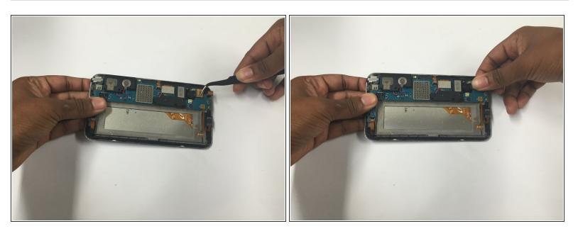
Gently put in the new rear facing and front facing camera and snap the tab back onto the motherboard.
