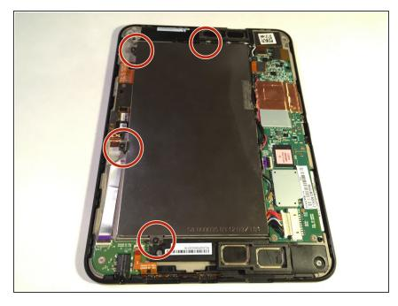
Locate the 4 Phillips #00 screws and use the Phillips head screwdriver to unscrew them.
