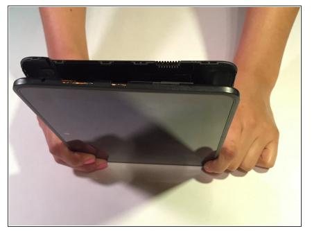
Using the plastic opening tool, start from one corner and go around the Kindle Fire using the tool in a down and up motion to continue to pop off the backing.
