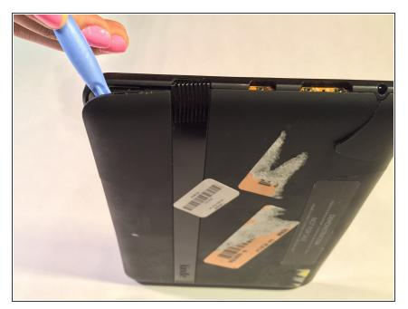
Using the plastic opening tool, carefully insert the opening tool on all four corners of the Kindle Fire and lift up until you hear a slight popping noise
