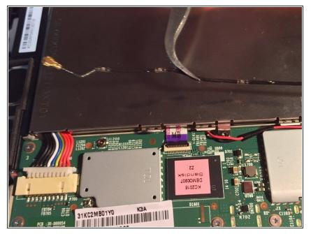
• Lift and pull up the power connector cable that surrounds the battery
