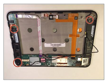
Look at the speakers on the left and right side of your device. Unscrew the three 2 mm screws that hold the speakers down with the Phillips #000 screwdriver.
