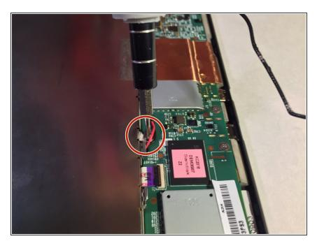
Locate the 1 T5 Torx screw and unscrew it.
