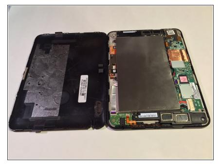
Once all the plastic clips holding the screen to the plastic back of the Kindle Fire are separated, the back should be safe to lift up completely.
