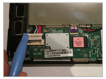
Use the plastic opening tool to remove the plastic piece that connects the wires to the motherboard
