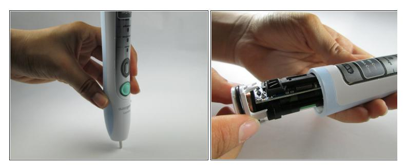
• Apply pressure to the shaft by pressing it against a firm and flat surface. Continue to apply pressure until the electronics located in the interior are exposed.
