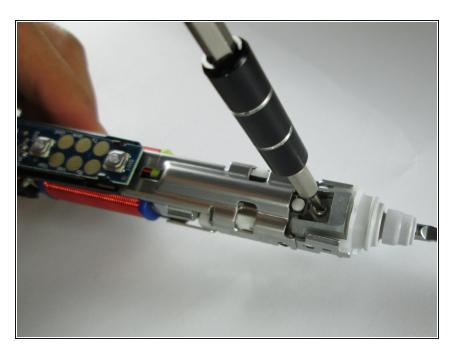
• Using a #00 phillips head screwdriver, loosen the screw completely.
