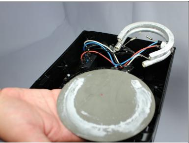
Push the heating plate up from below and remove.
