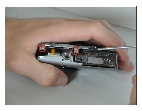
Remove 2 2.4mm screws on bottom.
