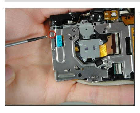
Remove one 3.9mm screw from inner frame.
