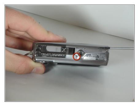
Remove one 2.25mm screw on the bottom.
