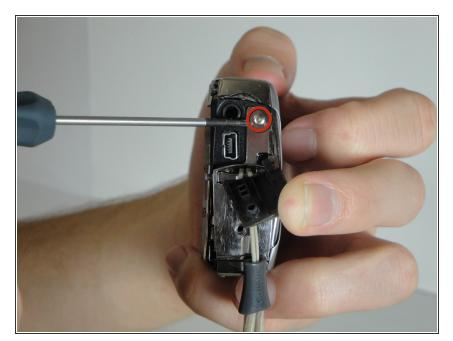
Remove the 3.9mm screw in the AV housing on the left side from the front of the camera.
