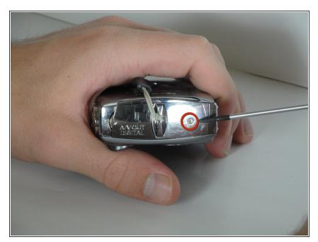
Remove one 4.7mm screw on the side with the AV output.
