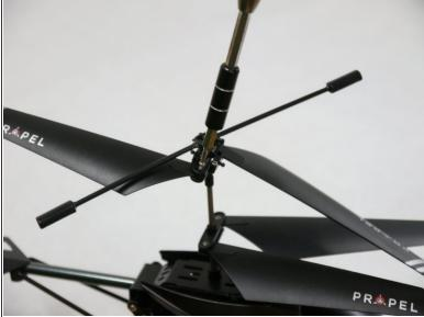
Remove the two 6.0 mm Phillips #00 screws from the rotors.
