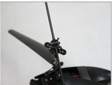
Pull the rotors away from the mounting brackets.
