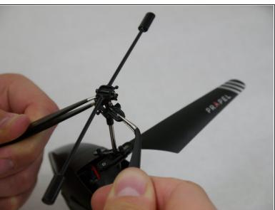
Using the tweezers twist the rotor attachment bracket apart.
