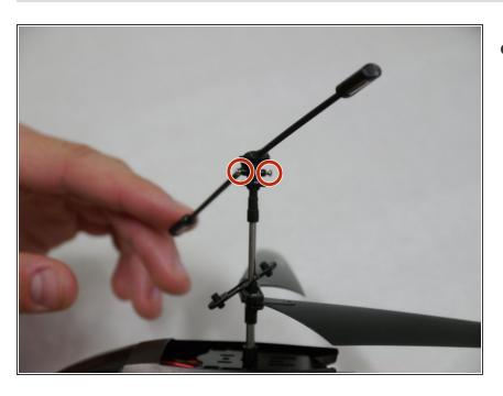
Remove the two 6mm #00 screws
