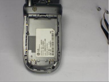
Use a Phillips #00 screwdriver to remove all four 3mm screws from the back of the phone.
