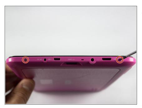
Use a screwdriver to remove the two 00 Phillips screws on the right side of the tablet.
