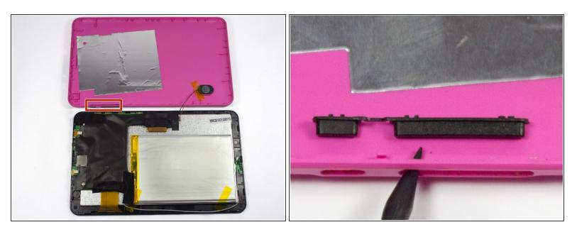
The buttons are located on the bottom left hand corner of pink back plate. Simply pop old buttons out with spudger or similar tool.
