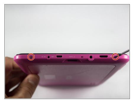
Remove the two 00 Phillips screws located in the right hand side of the tablet.
