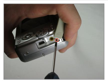
• Uncover the mini-usb dock on the side of the camera and unscrew the screw next to the flap joint
