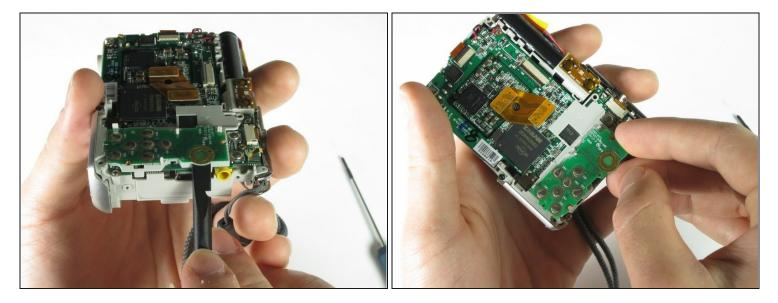
• Use the spudger or your fingers to remove the outer circuit board from the camera.
