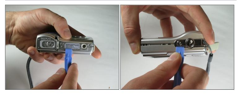
• Carefully slip the head of the plastic opening tool under the panels by finding the crack between the panels. Lightly apply pressure in the shown places at the top and bottom of the camera.
