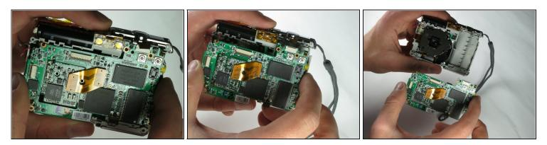
• Gently pull the motherboard (from the bottom first) away from the device.
