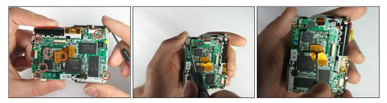
• Remove the screws shown using the 00 philips screwdriver.
