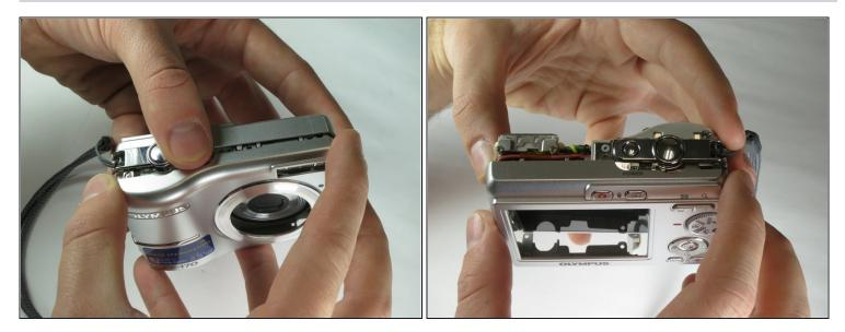
• Ensure that the panels have been loosened. Carefully use hands to pull back and remove the panels.
