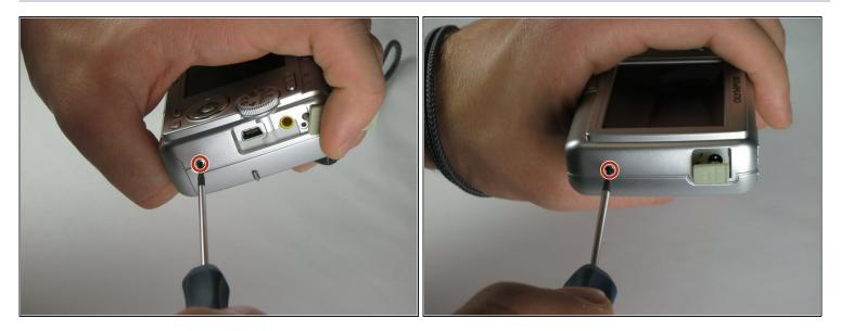
• Remove the 2 exposed screws on opposite sides of the camera. Turn the screws counterclockwise to remove.
