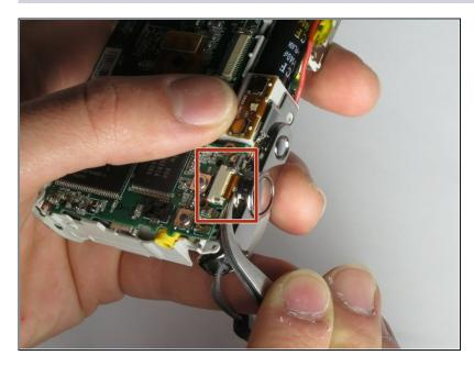
• Use the tweezers to remove the ribbon cable near the shutter button.
