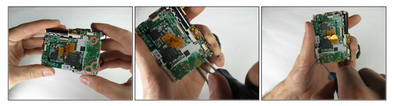
• Remove the three screws holding the outer circuit board in place.
