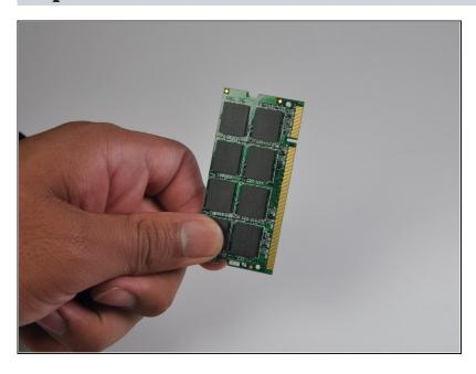
• Replace the RAM chip with a new RAM chip.
