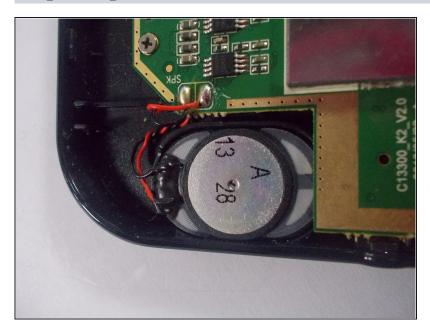
• Locate the two speakers on either side of the device
