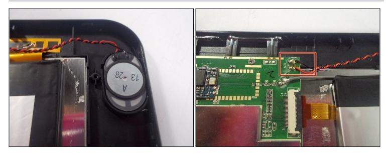
• Carefully disconnect the black and red wire from the motherboard using tweezers
