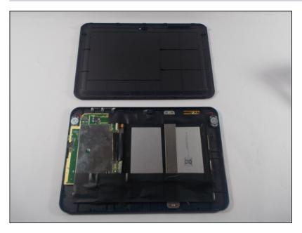
The back cover should then be able to easily be removed from the device and you should see the battery and other internal components.
