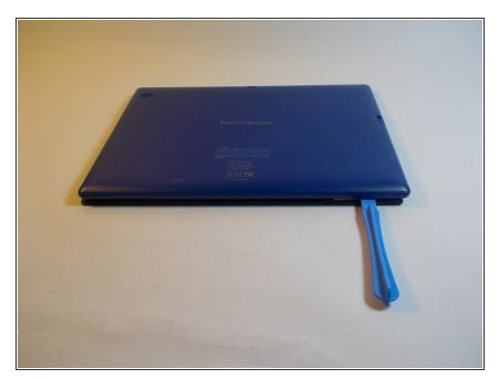
Place the plastic opening tool between the front and rear cover and pry up on each corner of the cover.
