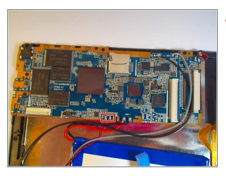
Melt the solders with a heat gun and remove red and black wires.
