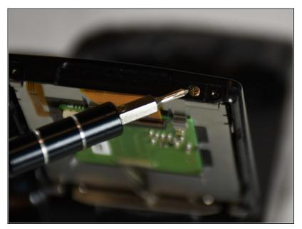
Unscrew the 2mm screw on the outer edge of the panel
