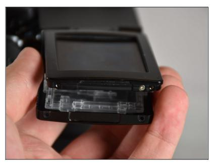
Pull off the back panel of the LCD screen and the plastic wire protector. Then replace the back panel.
