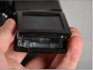
• Using the plastic opening tool, remove the rear case of the front LCD cover.
