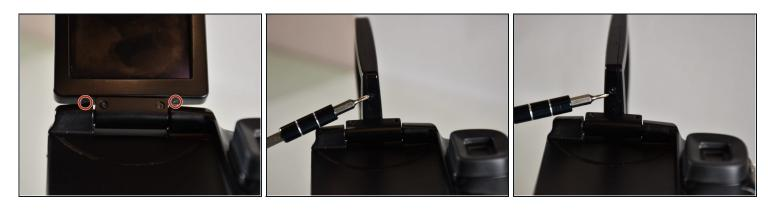
• Unscrew the two 3 mm screws shown on the right side of the LCD screen panel.
