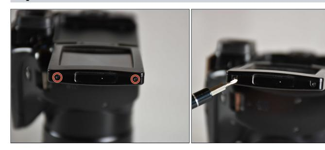
• Unscrew the two 3 mm screws shown on the left side of the LCD screen panel using a Phillips screwdriver.
