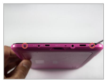
Remove the two 00 Phillips screws located in the right hand side of the tablet.
